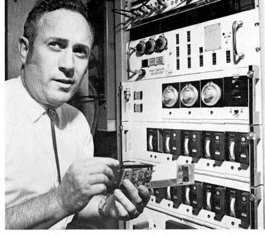
SPACE SAVER—These two banks of electronic tracking filters take the place of the nine racks of equipment previously required to obtain distance data during rocket tests. The array of filters was designed by Murray Silverman (9222) and will yield data from as many as 32 rockets.
